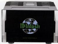
The power module (left) provides the actual amplification for the speakers. Two power modules are required to drive each speaker. One amplifies the positive half of a sound wave, the other amplifies the negative half. This arrangement is called fully complementary or balanced amplification. It helps cancel out noise, and it also allows the amplifier to swing from full positive to full negative more quickly.
