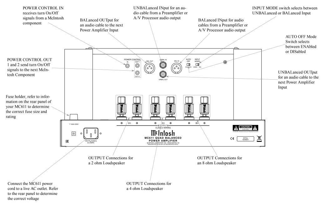
Caution: The Loudspeaker  $\bigcirc$  Negative Connections are above chassis ground. Do not combine any connections together, ground them or connect with another MC611.
