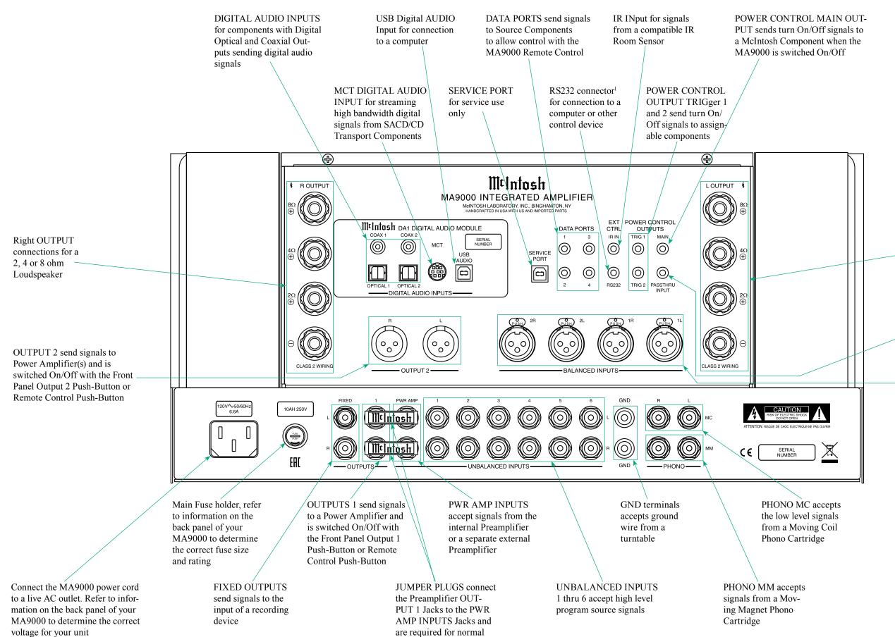
Left OUTPUT connections for a 2, 4 or 8 ohm Loudspeaker
