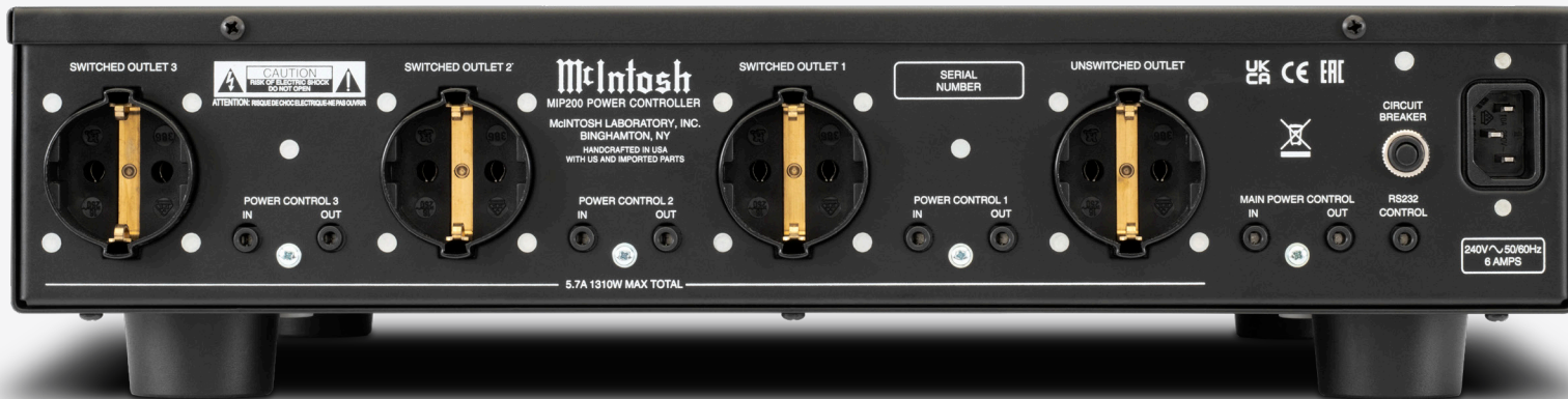
The MIP200 is available with either 4 Type B (NEMA 5-15R) outlets with 2 receptacles each (above), or 4 Type F (CEE 7/3 or “Schuko”) outlets with 1 receptacle each (below).
