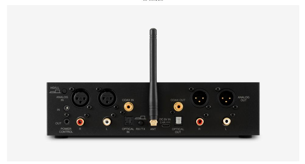
ABUNDANT CONNECTIVITY Remarkably versatile, the MB25 features an array of inputs and outputs to allow for diverse system configurations. Analog connectivity options include both balanced and unbalanced stereo inputs and outputs.
